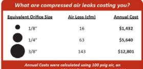
Annual Costs were calculated using 100 psig air, an average energy rate of \$0.080/kWh, and assuming 6,000 annual operating hours and 4.0 cfm/bhp
